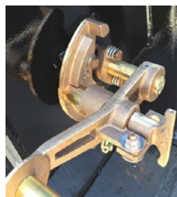
Figure 11. Switch-Handle Packing Gland
