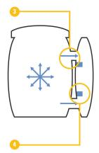
Radiator Spacer Failure allows "pillowing", creating large expansion volume
