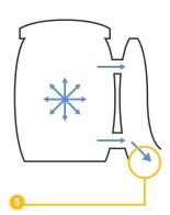
Radiator designed to fail at bottom or side serving as a directional blowout port
