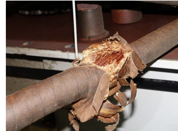
Tap Lead Insulation Damage
