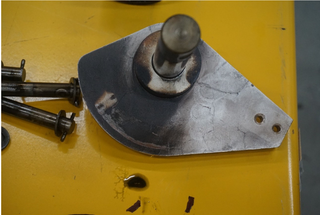
Reversing Switch Isolated Neutral: Heating & Carbon Buildup
