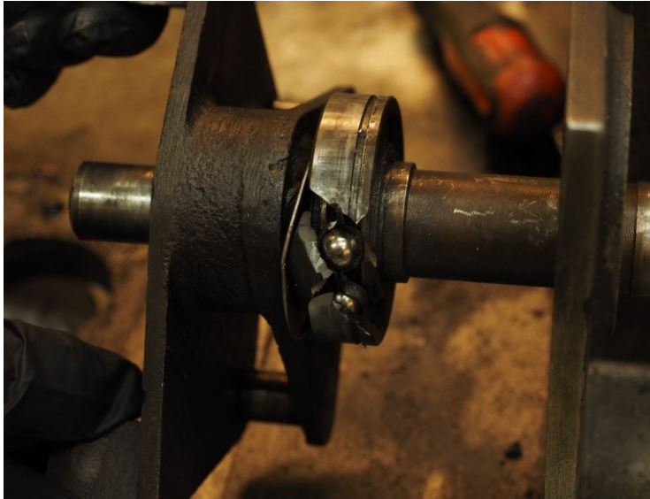
Shattered Bearing on First Shaft Assembly
