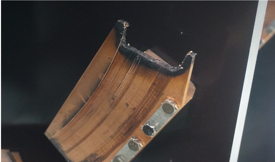
Selector Switch Stationary Contact with Severe Arcing Damage
