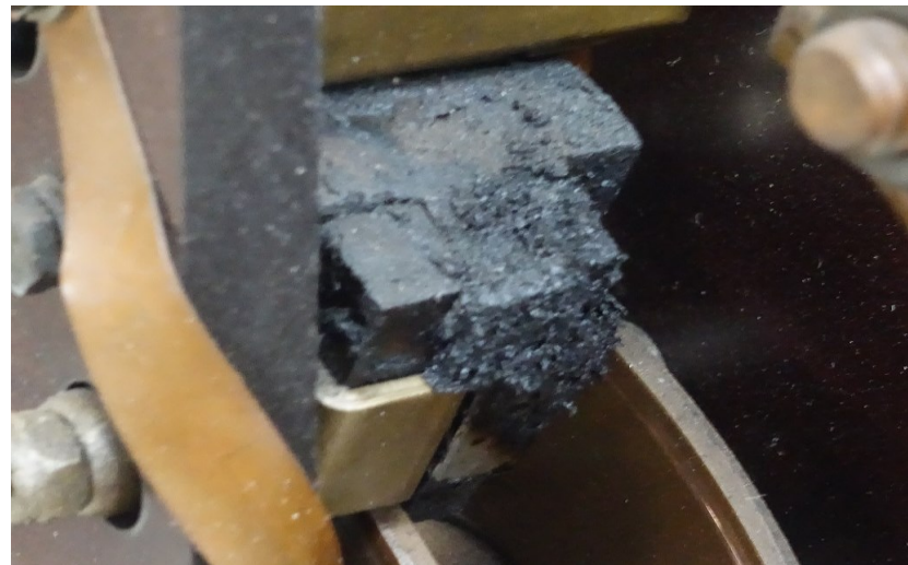
Tap Lead Insulation Damage
