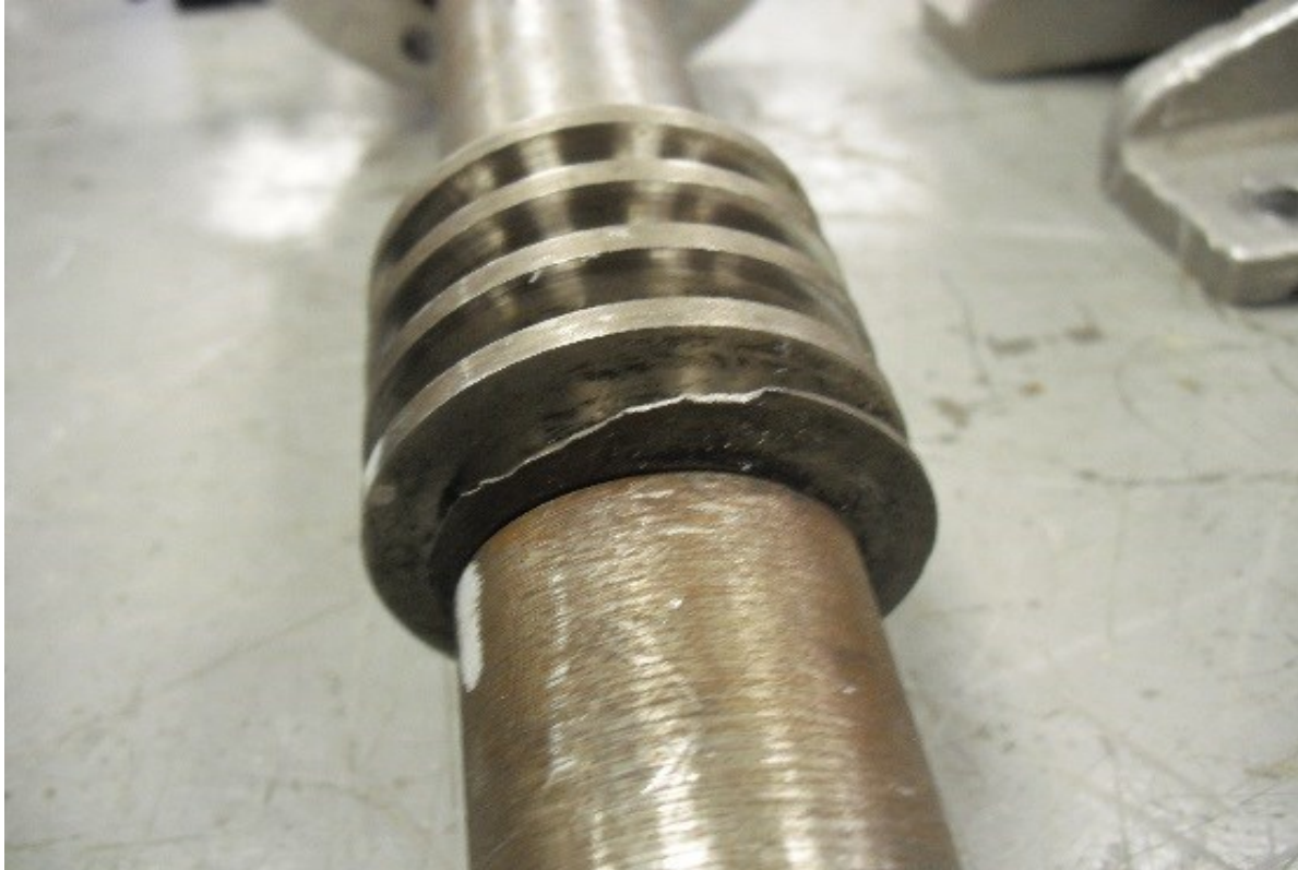
Vertical Worm Gear Drive Shaft Damage
