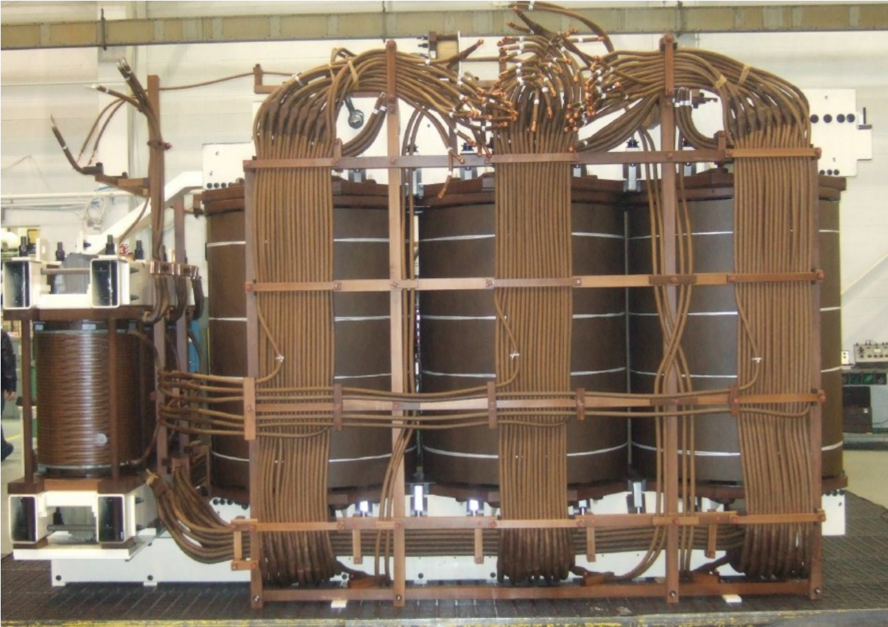
LTC Lead Connections – Multi Start Windings
