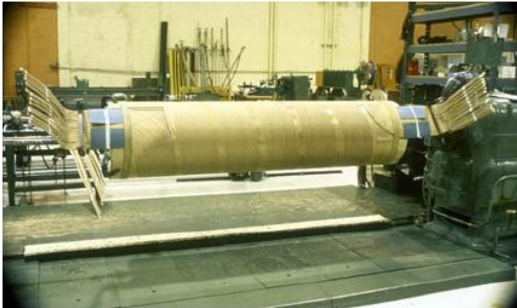
Regulating Voltage Winding Design
