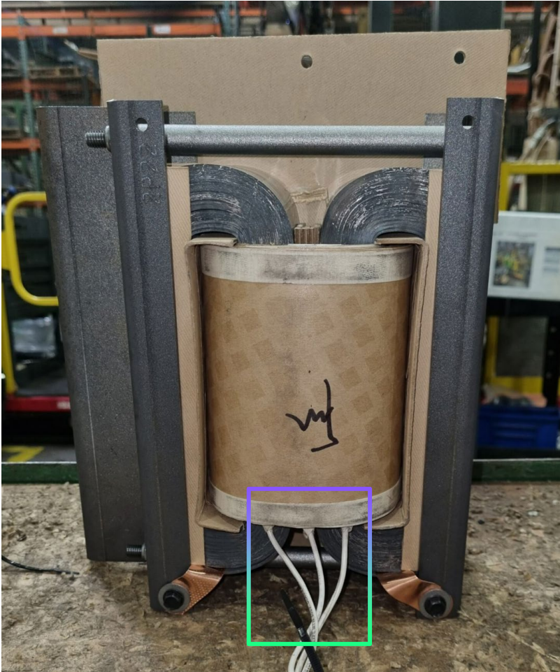
Low Voltage Taps
