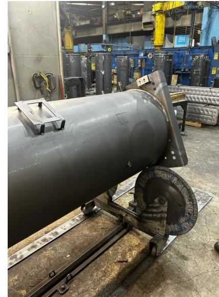
Tank is welded to the base
