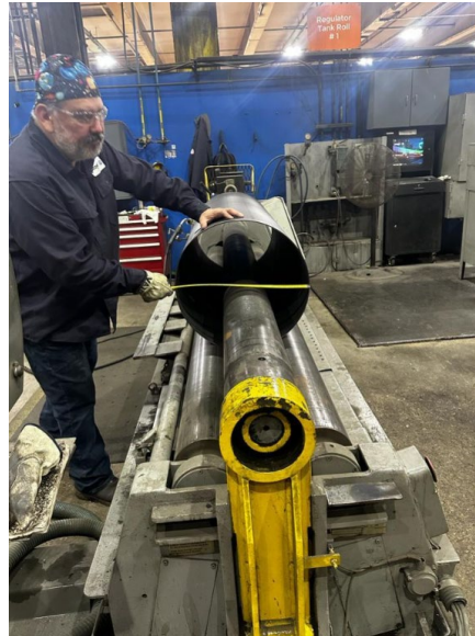
Diameter of the tank is measured
